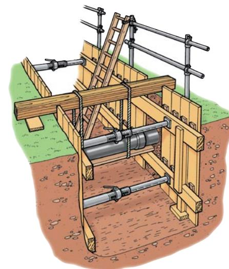
**Figure 44** An excavation supported by timbering and props with guard rails (omitted from left-hand side for clarity) to prevent falls. Extended poling boards act as toe boards, safe access is provided by a tied ladder and exposed services are supported
