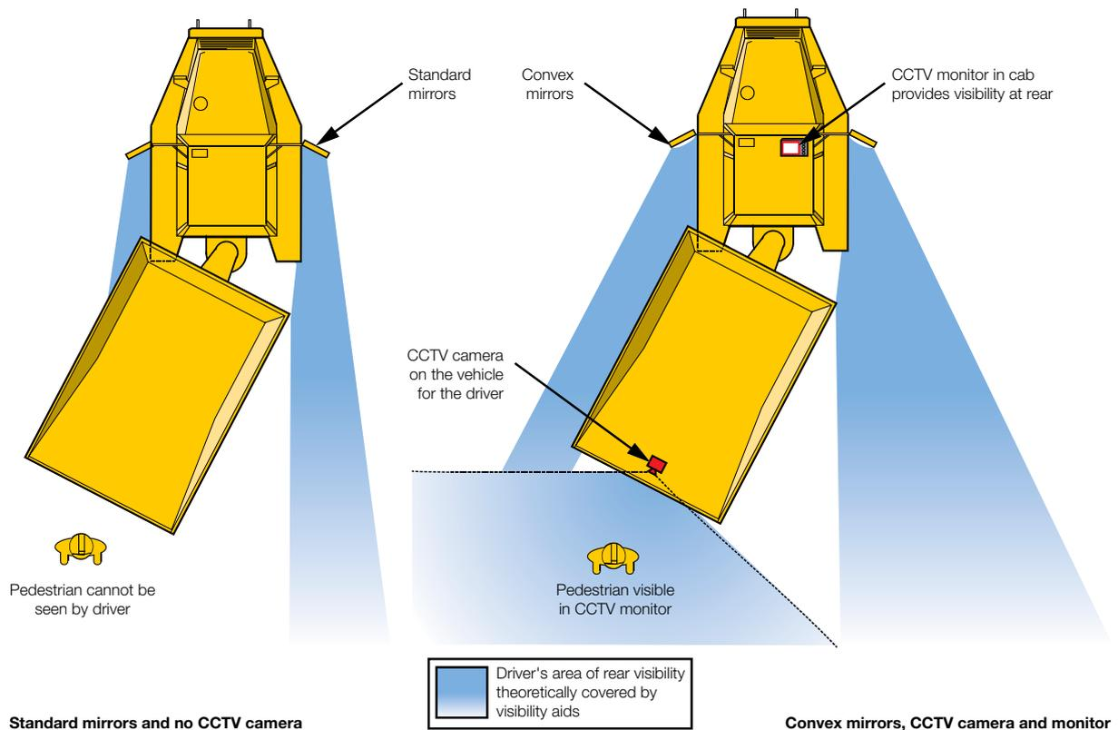
**Figure 37** Some vehicles are fitted with vision aids such as mirrors or CCTV, which help drivers to see areas that they cannot view directly
