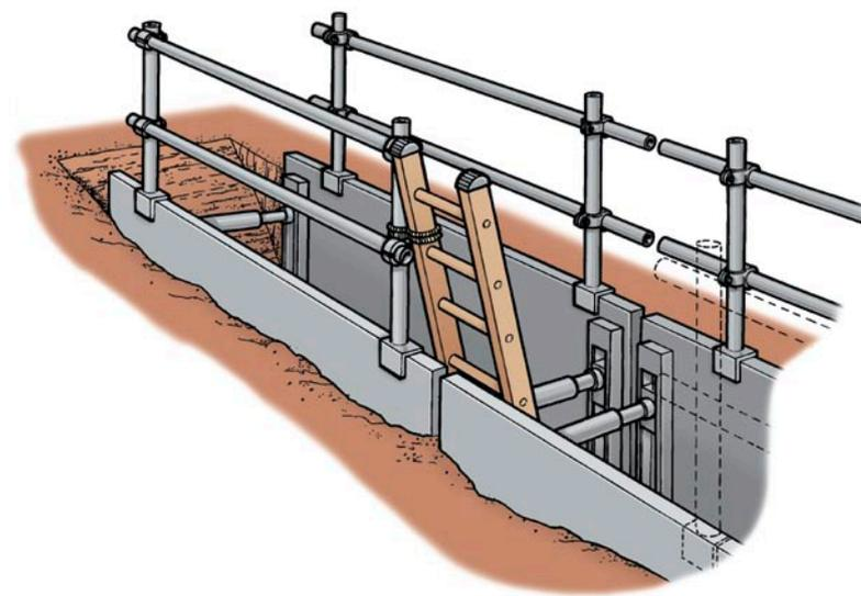
**Figure 43** A trench box with guard rails attached
