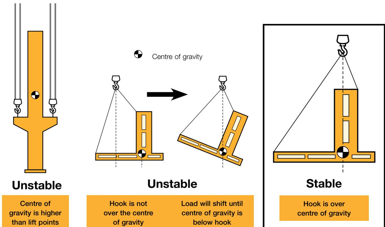
Figure 41 The centre of gravity must be beneath the hook
