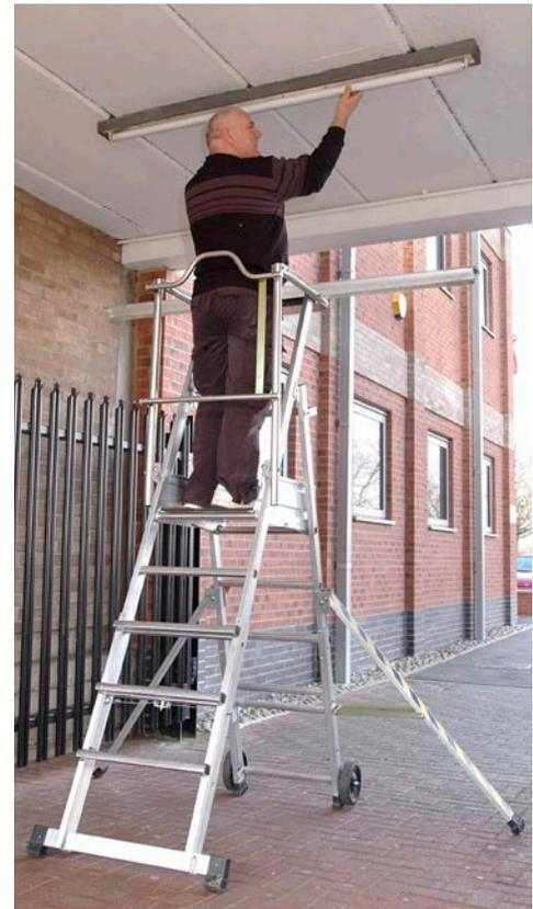
**Figure 22** Working platform stepladder
