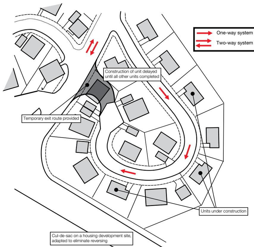
**Figure 32** Provide drive-in/drive-out access to delivery and work areas
